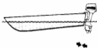
INSUFFICIENT ANGLE (Bow digs)
