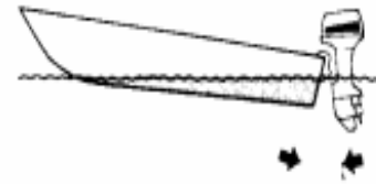
EXCESSIVE ANGLE (transom drags)
